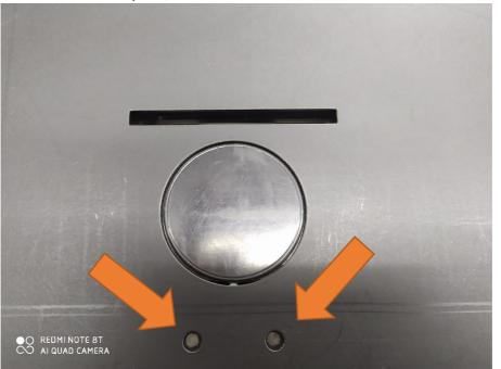
3. Re-Position the Mover manually at the Park-Position by **carefully/slightly moving/pushing** it. Because of the **magnet inside the Stage** should always re-locate and re-align the Mover at the correct position and angle.
