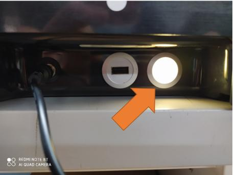
2. Check that the **two tiny sensor-openings/holes** at the Park-Position of the Stage are neither soiled nor blocked by **dirt/dust**.
