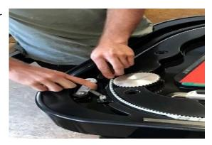
When installing the new drive belt the magnet cam has to be installed behind the mover park position as shown in the photo. The magnet cam must not be inserted directly in the park position as the limit switches may bedamaged.
