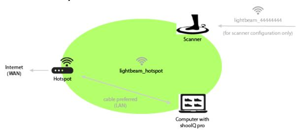
The scanner must be in the same local network as the computer with the shoolQ pro software. Therefore we provide a preconfigured Hotspot with the SSID **lightbeam\_hotspot** with the scanner. The mover (robot) of the scanner is also preconfigured onto this SSID. Therefore you must only connect the hotspot to the internet via cable with the **WAN** port of the device and your computer by ethernet cable to the **LAN** port of the hotspot (or by WiFi with the **lig htbeam\_hotspot**).
