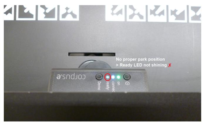
• If the Mover is not in the middle of the park position, please try to slightly move it by hand and see if the "Ready" LED is shining again
