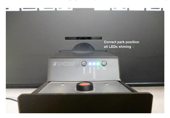
If the "Ready" LED on the Mover is not shining, please check if the Mover is properly in the park position
